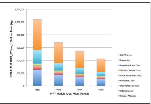
Figure 7-7 Impact of Variations in the Solar Power Generation Technology Ratio (D3/S1)
