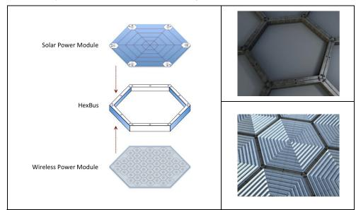
Figure 3-12 Illustrations of the SPS-ALPHA Primary Array Assembly (PAA)
