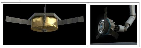
Figure 3-11 Illustrations of the "Propulsion / Attitude Control" (PAC) Concept
