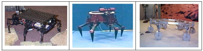
Figure 3-21 Several Generations of Hexabot Robots from the mid-1990s (Credit: NASA/JPL)
