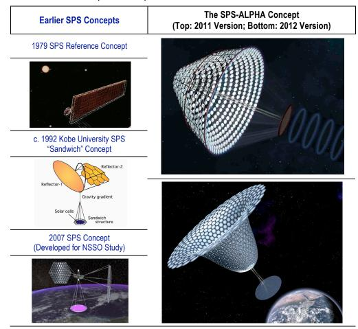
Figure 1-1 Selected Past Solar Power Satellite Concepts and 2 Versions of the New SPS-ALPHA Concept
