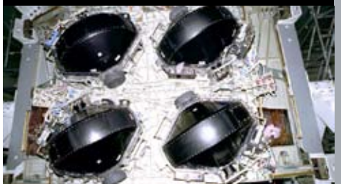
Control Moment Gyroscope gimbals used for orienting the ISS.
