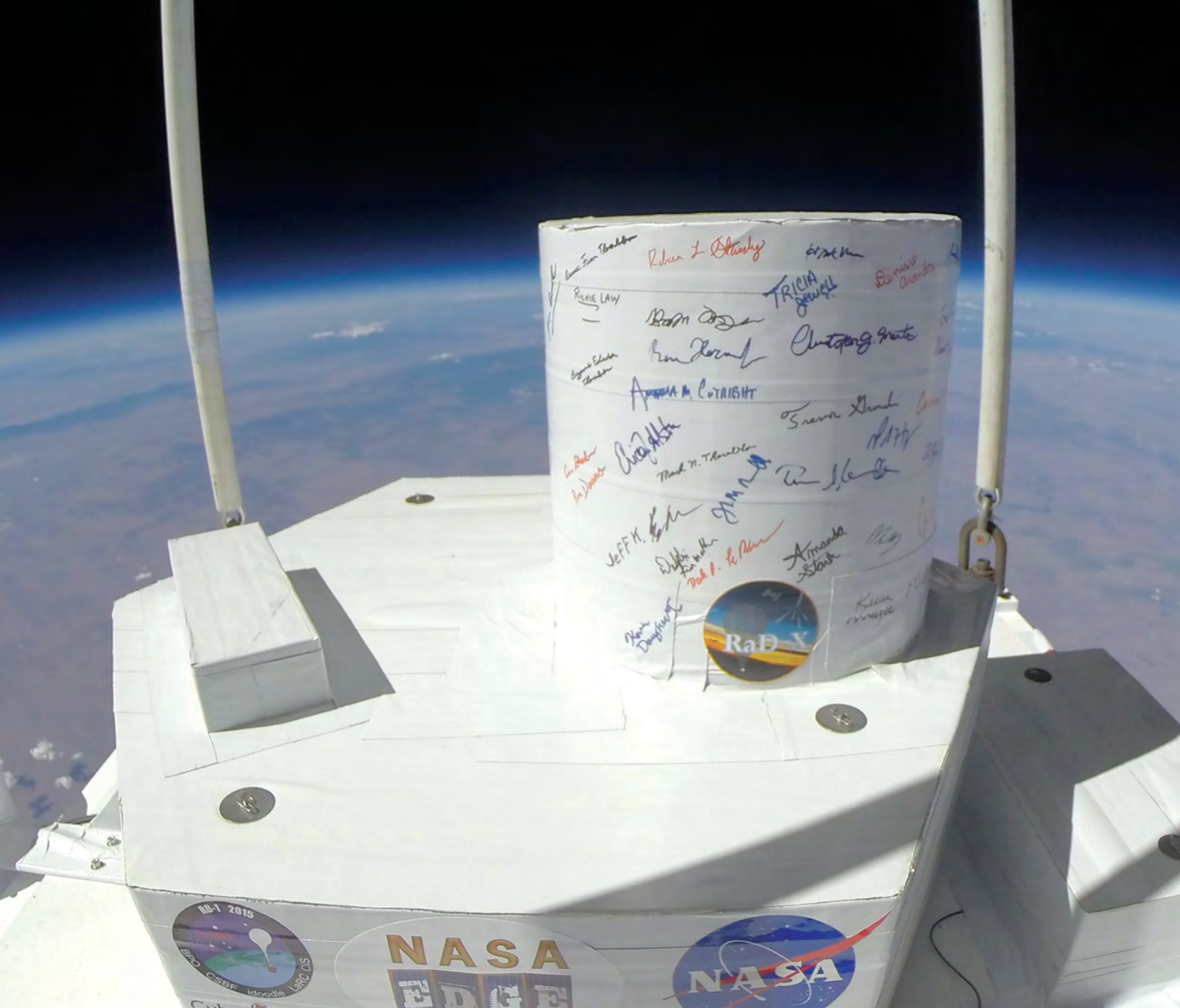
NASA's Rad-X experiment flew aboard a high altitude balloon to measure radiation doses over time. Credit: NASA
