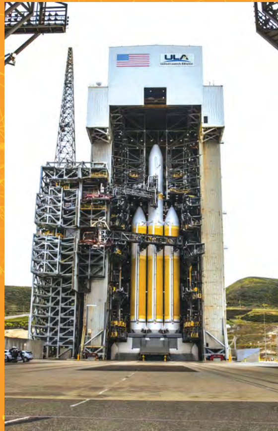
A United Launch Alliance Delta IV Heavy inside the servicing structure Credit: ULA
