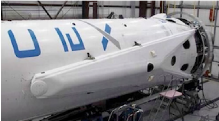
Above: legs folded against sides of booster
