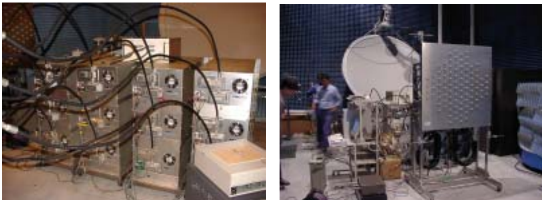
Fig.3.2 Phased Array with 2.45GHz Phase Controlled Magnetrons Developed in Kyoto University
