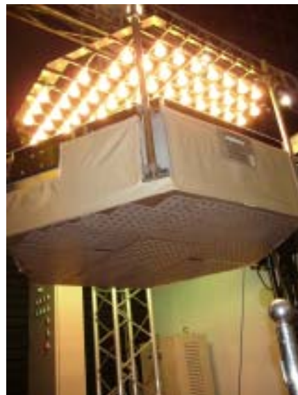
Fig.3.1 Phased Array Used in Japanese Field MPT Experiment (Left : for MILAX in 1992, Right : for SPRITZ in 2000)
