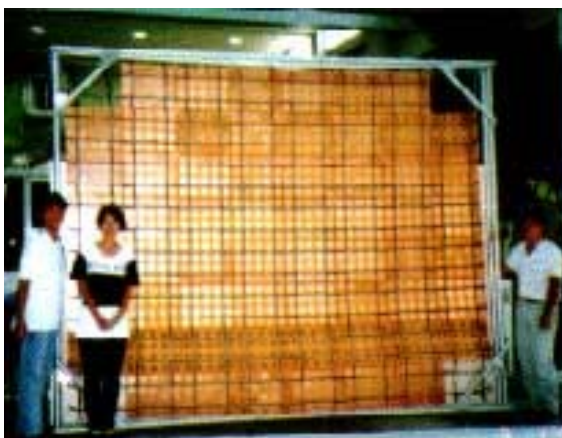
Fig. 5.3 Large Rectenna Array Used for (a) G-to-G Experiment in Goldstone in 1975 [27], (b) G-to-G Experiment in Japan in 1994-95 [28], (c) fuel-free airship experiment in 1995 [10], (d) Experimental Equipment in Kyoto University [29]
