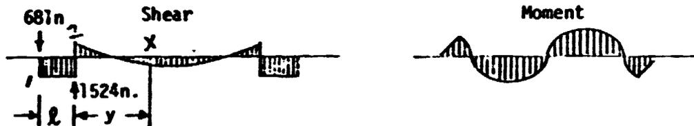
The moment from point 1 to 2 is  $681l$  and is equal to  $555.875$  n-m at point 2. The moment from 2 to X peaks at  $1.25 \times 10^6$  n-m at  $y = 5000$  (halfway between the center and end of the blanket).
