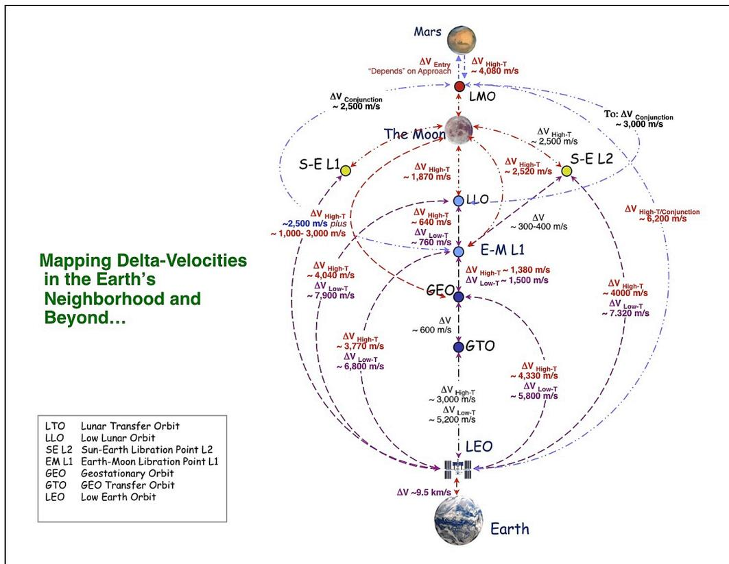
Figure 6-3 Space Transport Energy Requirements Diagram
