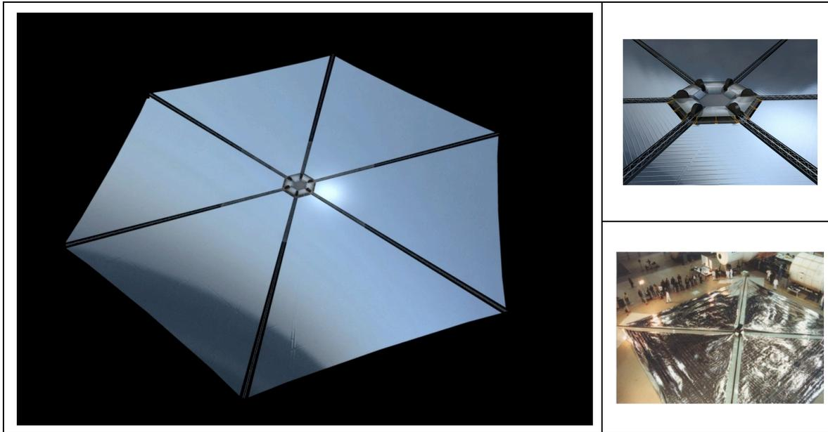
Figure 3-13 Illustrations of the SPS-ALPHA Solar Reflector Array
