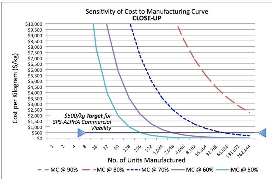
Figure 4-4 Close-Up View of a Portion of Figure 4-3
