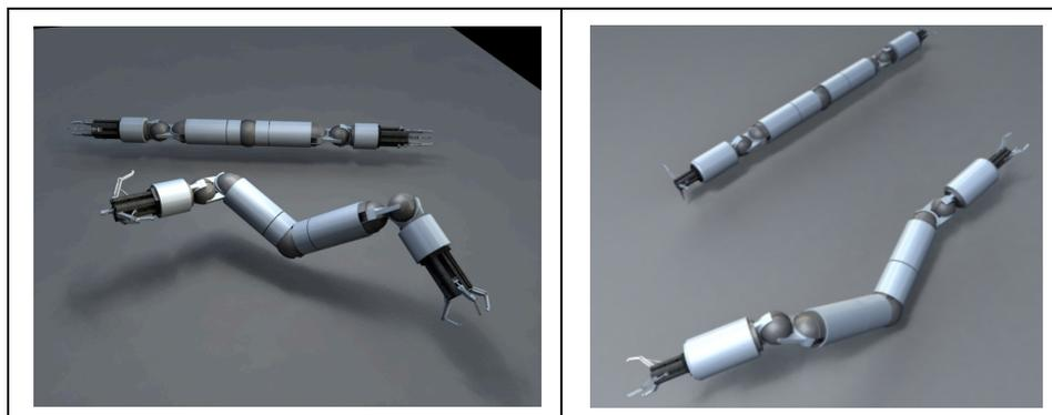
Figure 3-10 The Modular “Push-Me/Pull-You” Robot (MPPR) Arms Concept
