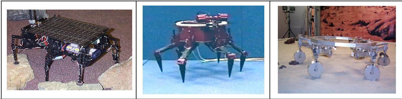
Figure 3-21 Several Generations of Hexabot Robots from the mid-1990s (Credit: NASA/JPL)
