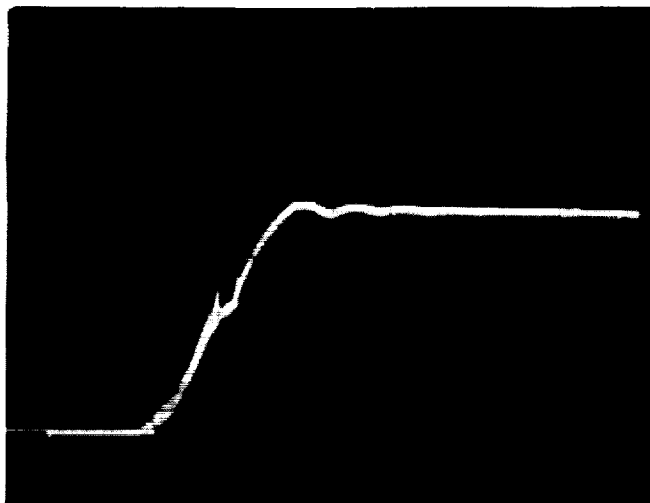
Figure 3-1. Transient Starting Behavior of Magnetron Directional Amplifier.
