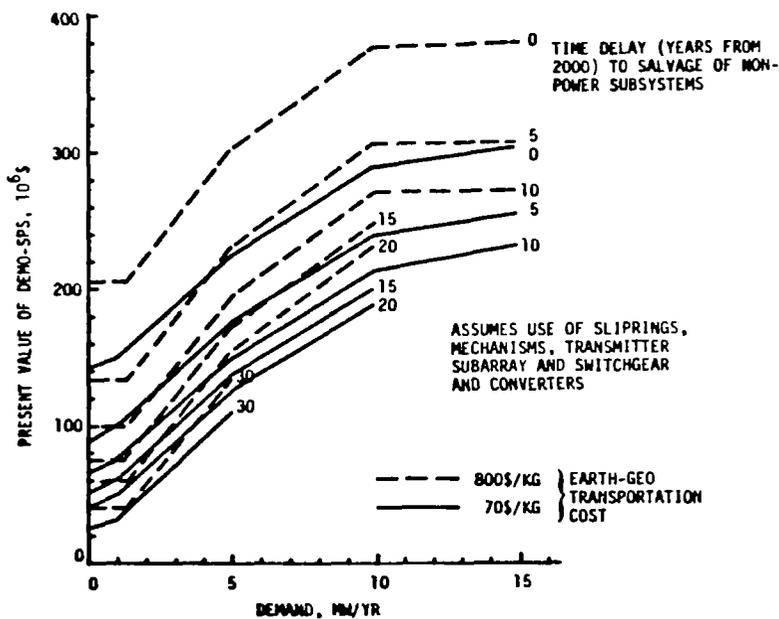
FIGURE 3.8 SALVAGE VALUE OF SPS DEMONSTRATION SATELLITE WHEN USED AS A SOURCE OF POWER AND OTHER SUBSYSTEMS FOR OTHER ACTIVITIES (GEO PLATFORMS, MANUFACTURING BASE, OTV OR SPACE EXPLORATION VEHICLES)
