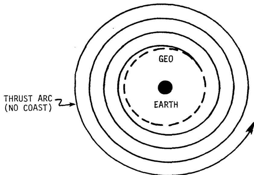
(a) CONTINUOUS THRUST SPIRAL TRAJECTORY MODE
