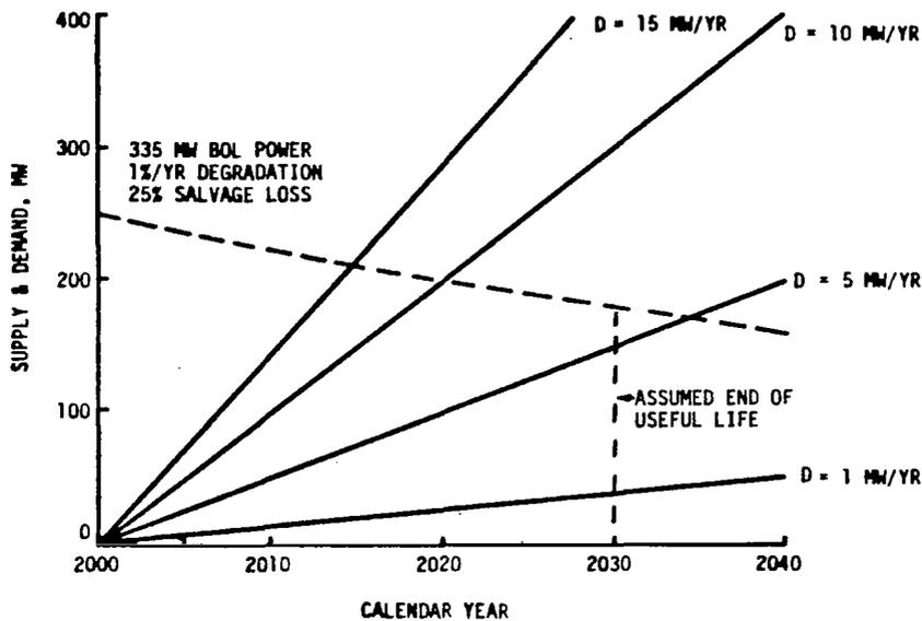
FIGURE 3.5 SUPPLY & DEMAND FOR POWER FROM DEMONSTRATION SPS SATELLITE
