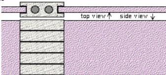
Panels, whether of concrete or made in the same moondust sintering fashion as bricks and blocks, could be held in place by Lego type blocks with forked ends.
