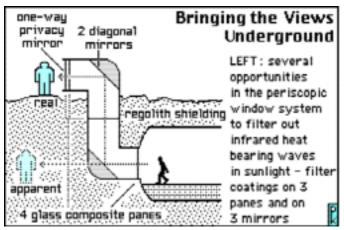
RESEARCH: Now the "Z-View" periscopic window assembly looks simple in principle. With the zigzag light-path, radiation protection is preserved. The interior air-pressure could be stepped down gradually, by one or two transparent panes, placed at intervals.
