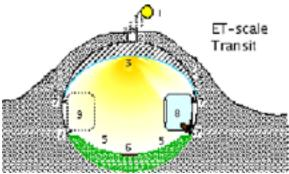
**KEY**: (1, 2, 3, 5, 6) as above. (7) wall-mount rail suspension system, (8, 9) bench seat transit car.
