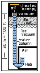
The weight of column of water 30 meters or 100 feet high exerts enough counter-pressure to keep habitat atmosphere at 0.5 Earth normal (42% O2, 58% N2) pressure from flowing out the open ended J-shaped tube.
