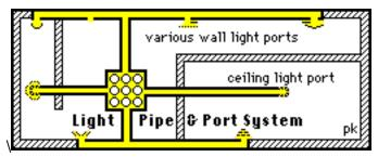
Wall and Ceiling Light Ports could then be fitted with any of a growing choice of consumer purchased and artist designed decorative plain, etched, or stained glass; or pierced metal diffusers; or fiberglass fabric shades. Such a system might allow the number of types of bulbs that need to be manufactured to be minimized, allow the use of the most efficient bulb types, appreciably reduce the amount of wiring needed, and still allow wide decorator choices. **MMM**
