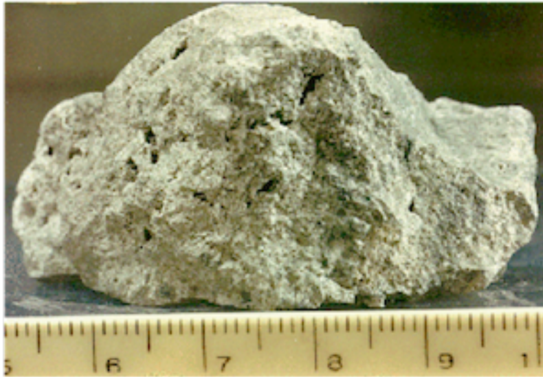
This 5" long rock is rich in KREEP: Potassium (K), Rare Earth Elements (REE) and Phosphorus (P)
