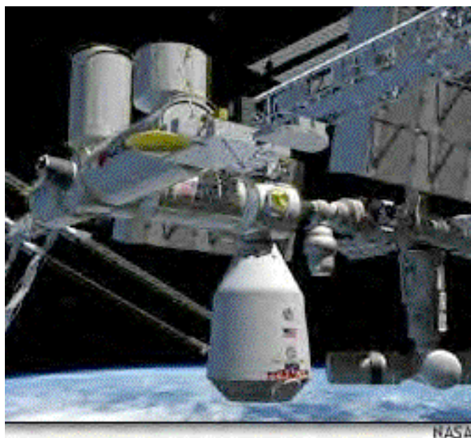
A NASA-JSC illustration of an ISS version of TransHab attached to the space station. The evident teardrop shape seems to this writer to have been a case of artistic license that makes no sense at all and implies that a hard shell had
