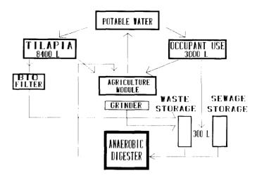
Fig. 1. Theoretical flow chart of wastes and water in lunar base CELSS.
