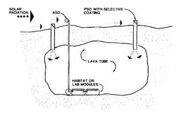
Fig. 5. Operational base using ASO and PSO.
