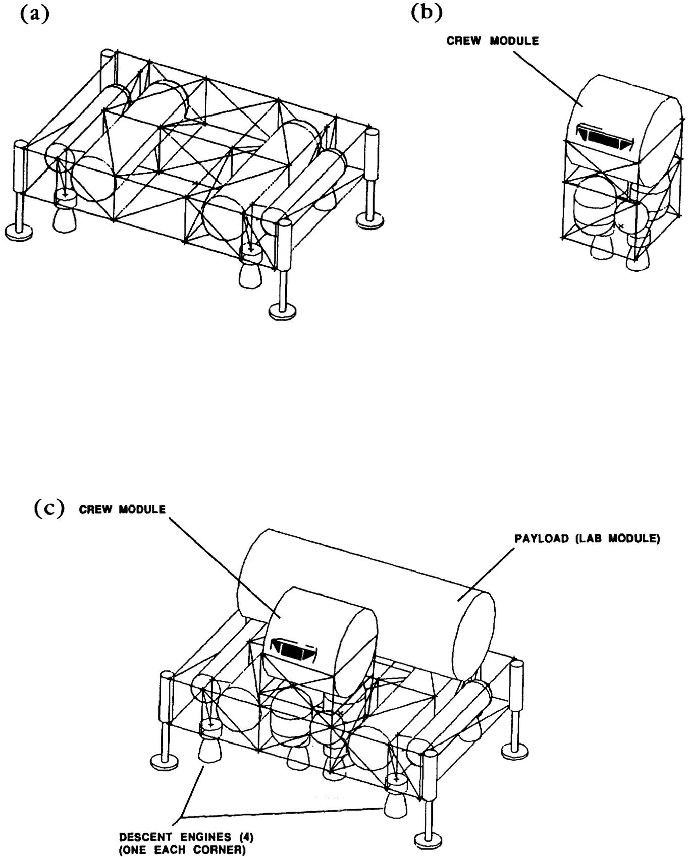
Fig. 11. Lander stage configuration. (a) descent stage (expendable or reusable); (b) ascent stage (expendable); and (c) descent stage with ascent stage plus payload.
