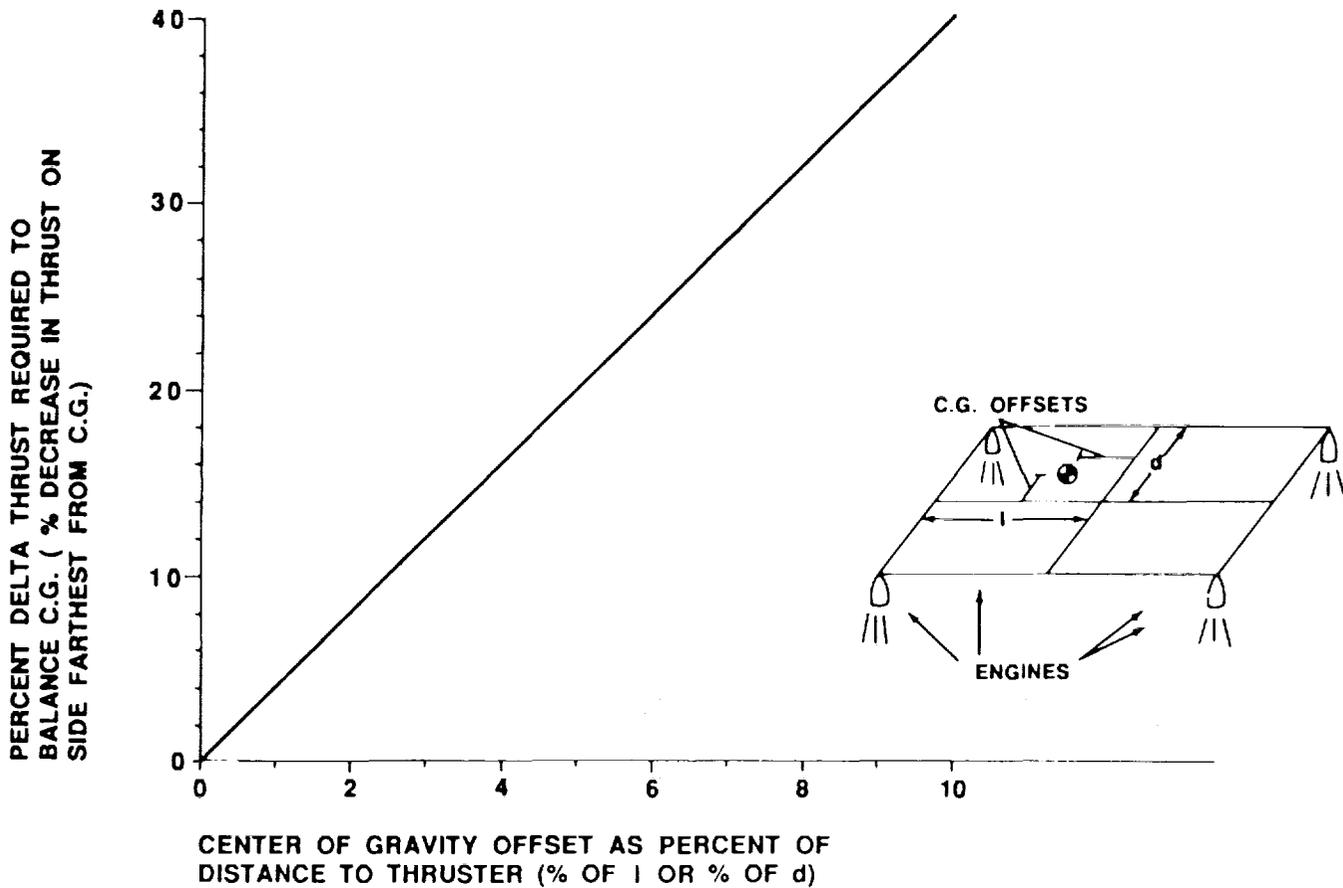
Fig. 10. Throttability required to balance center-of-gravity offsets.
