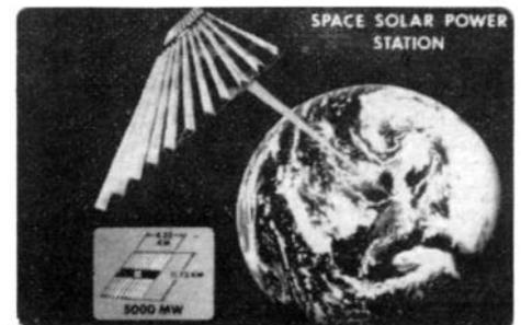
303 Photovoltaic type of solar power satellite with one km. diameter transmitter/antenna in center (Arthur D. Little design).
