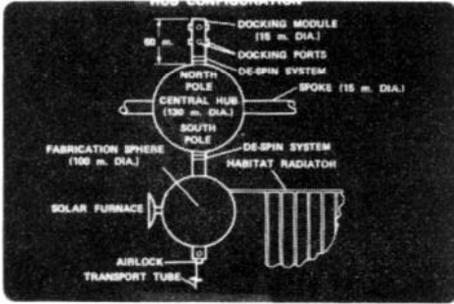
227 Details of the Stanford Torus design -- hub configuration.
