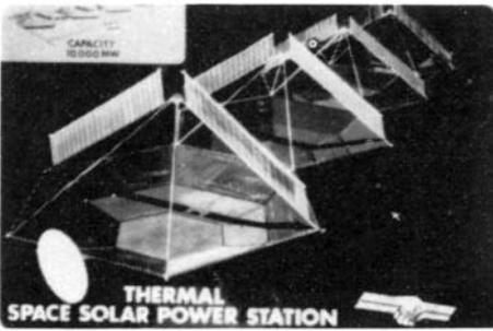
307 Photo-thermal type of solar power satellite, white disk is the transmitter/antenna (Boeing).
