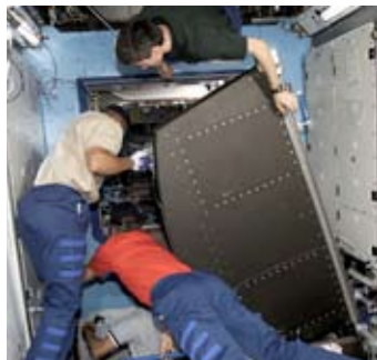
Crew installs a rack in the U.S. Lab in orbit.
