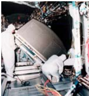
Installation of a rack in the U.S. Lab prior to launch.
