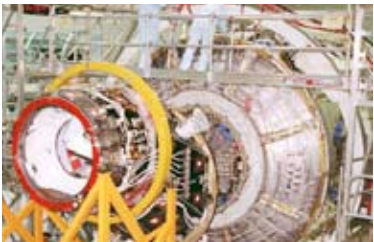
PMA 1 is being attached to the Common Berthing Mechanism of Node 1.
