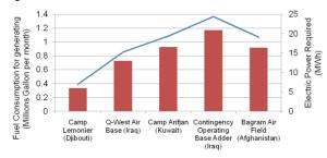
Fig. 5. Power Required For US Forces in Forward-Deployed Regions. Note: Electric power required is calculated using fuel consumption of 4 gallon/hour for a 60 kilowatt generator.<sup>15</sup>
