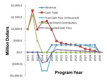
Fig. 9. SSP FRS: Firm Revenue and Cost Flows for Govt. DDT&E Contribution Case (Government Contribution = 100% DDT&E, Equity Investment = \$300M total during acquisition, Break-Even Price = \$7.18 /kWh)
