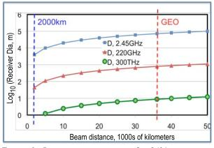
Figure 1: Receiving antenna size for 84% capture vs. beam distance
