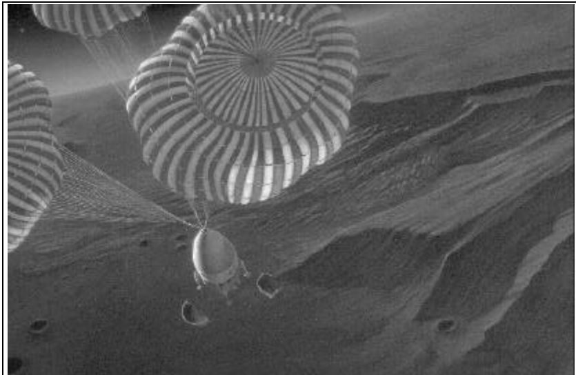
Figure 2.2-1 The transit habitat vehicle with the first human crew descending on parachutes before using terminal descent propulsion. This vehicle will land in the near vicinity of the previously deployed surface assets—the ascent vehicle, the ISRU plant, the power plant, and other surface equipment not needed by the crew during the outbound journey.
