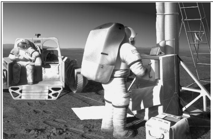
Figure 2.19-1 An EVA crew member changes a faulty line replaceable unit on one element of the surface infrastructure. EVA-accessible enclosures and compatible disconnects will be necessary to allow for effective use of crew time during maintenance and repair activities. (© Lockheed Martin)
