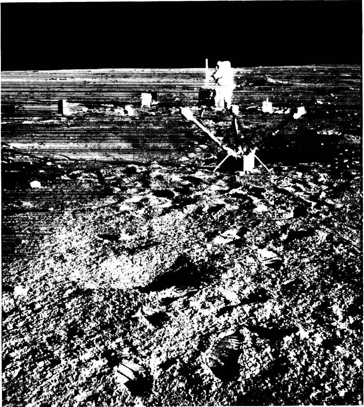
Figure IV-4. A proven way to deploy geophysical instruments is to use astronauts. An Apollo 12 crew member is shown setting up the ALSEP (Apollo Lunar Surface Experiment Package) central station, which contains data processing and transmission facilities. The passive seismic station is to the right, and the magnetometer is in the foreground.
