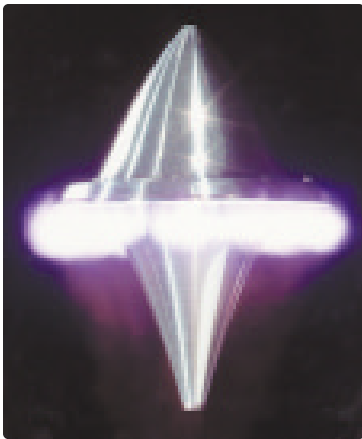
A model of a lightcraft, illuminated from below by a laser beam.
